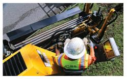
**NARROW FOOTPRINT.** With a slender profile of 44 in (111.8 cm) in width, the drill can easily maneuver within narrow jobsites and position side by side with a mix system on a trailer, helping to increase productivity when working in urban spaces.
