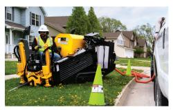
**COMPACT BUT POWERFUL.** The D10x15 S3 stands out due to its compact design and light weight. With 10,000 lb (44.5 kN) of thrust/pullback and 1,500 ft-lb (2,033.7 Nm) of rotational torque, it has the power required for tough ground conditions and pulling reamers.
