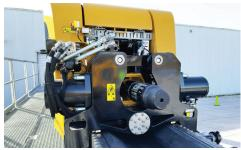
HIGH-CAPABILITY DRILL. With a maximum torque of 110 kNm, the D120E delivers the hole-making capability comparable to a larger maxi rig. The direct, electric drive results in reactiveness, controllability and scalability of the rig for highly efficient operations.
