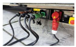
**DIFFERENT POWER SOURCES.** You can plug the drill to a genset or to the grid or to a battery pack. Regardless of the type of power source you have available on site, the D120E will perform.
