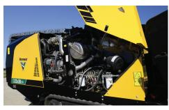
**PREMIUM POWER.** A 100 hp (75 kW) Deutz TCD3.6L4 engine provides power to help drive the D23x30DR S3 to its peak performance, while a thrust/pullback of 24,000 lb (106.8 kN) combines with rotational torque of 3,000 ft-lb (4067.5 Nm) to help get the drill into tough ground.
