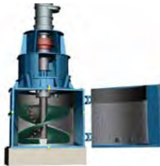
The bodies of Metso Vertimills are lined with Orebed®.
